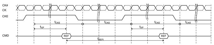
NOTE: The pattern shown above can repeat over a long period of time. With this pattern, DRAM guarantees all AC and DC timing & voltage specifications and DLL operation with temperature and voltage drift
