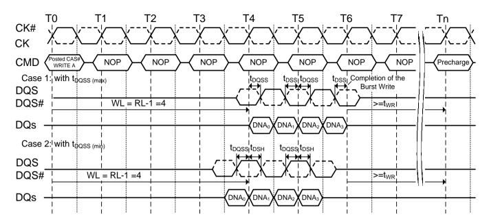
Figure 27. Burst write operation: RL=5 (AL=2, CL=3), WL=4, BL=4
