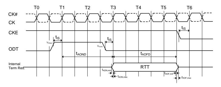
Figure 14. ODT timing for power-down mode
