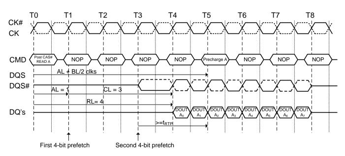
Figure 35. Burst read operation followed by precharge: (RL=5, AL=2, CL=3, BL=4, t<sub>RTP</sub> ≤ 2 clocks)
