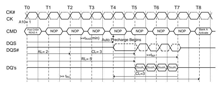
Figure 43. Burst read operation with auto precharge followed by an activation to the same bank (t<sub>RP</sub> Limit): (RL=5 (AL=2, CL=3, internal t<sub>RCD</sub>=3, BL=4, t<sub>RTP</sub>≤ 2 clocks)
