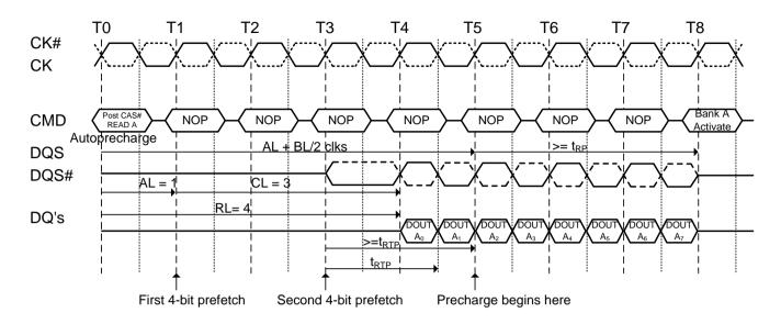
Figure 41. Burst read operation with auto precharge: (RL=4, AL=1, CL=3, BL=4, t<sub>RTP</sub> > 2 clocks)
