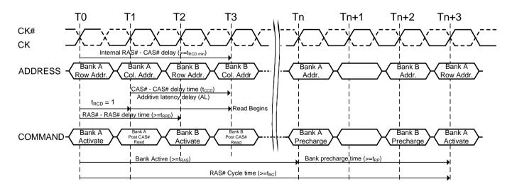
Figure 18. Posted CAS# operation: AL=2 Read followed by a write to the same bank
