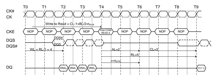
NOTE: The minimum number of clock from the burst write command to the burst read command is  $[CL-1 + BL/2 + t_{WTR}]$ . This  $t_{WTR}$  is not a write recovery time ( $t_{WR}$ ) but the time required to transfer the 4 bit write data from the input buffer into sense amplifiers in the array.  $t_{WTR}$  is defined in the timing parameter table of this standard.
