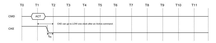
Figure 57. Precharge/precharge-all command to power-down entry
