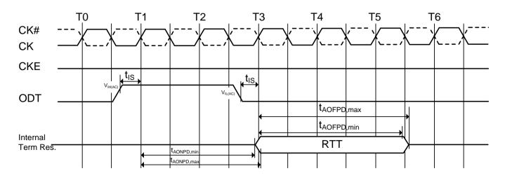
Figure 15. ODT timing mode switch at entering power-down mode
