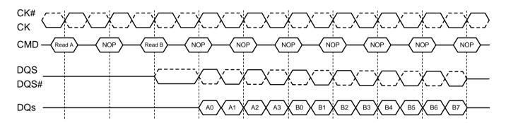
NOTE 1: Read burst interrupt function is only allowed on burst of 8. Burst interrupt of 4 is prohibited.
