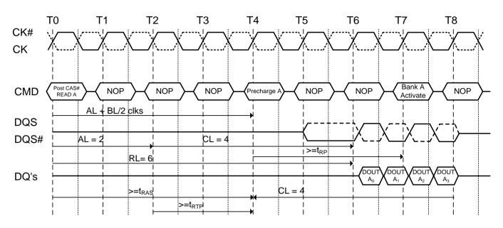
Figure 37. Burst read operation followed by precharge: (RL=4, AL=0, CL=4, BL=8, t<sub>RTP</sub>>2 clocks)
