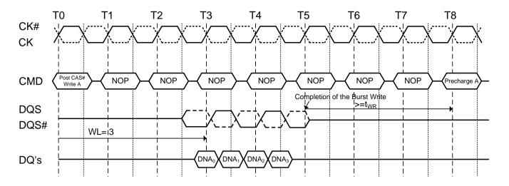
Figure 39. Burst write followed by precharge: WL= (RL-1) =4
